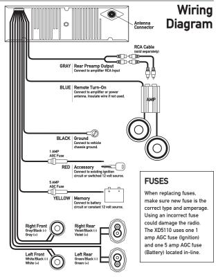
\* CAUTION - Do not attach any speaker leads to ground as severe damage will occur.
